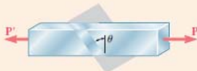
Fig. 1.46 Axially loaded member with oblique section plane.
